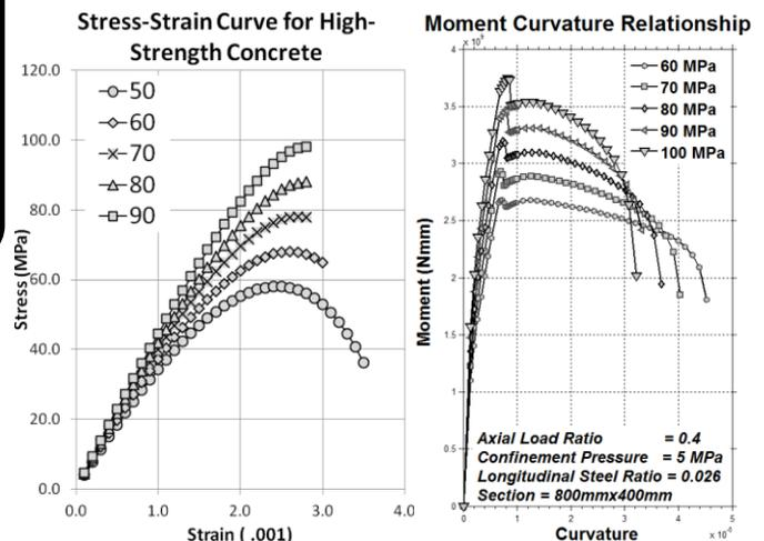
Figure 02: Brittleness of HSC and Ductility of HSC column
